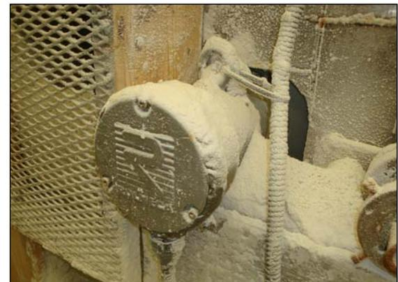
*Salt cannot penetrate oil-filled pulley shell.*
