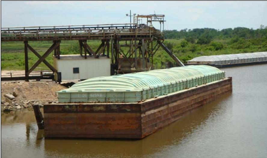
*One of two barge loader conveyors now driven by Rulmecca Motorized Pulley at Cargill Deicing salt mine and barge loading terminal in Avery Island, Louisiana*
