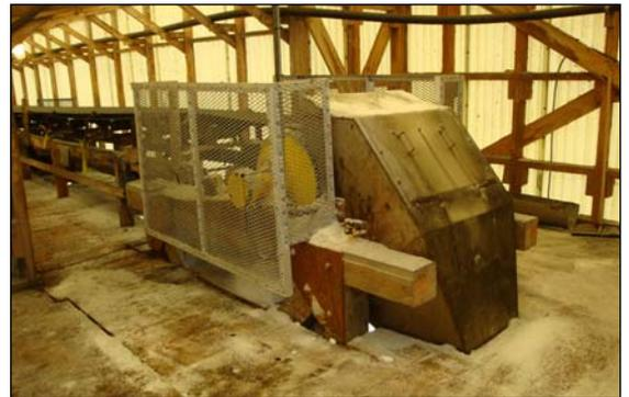
*Note compactness of 60 HP internally-powered hermetically sealed Rulmecca Motorized Pulley drive.*
