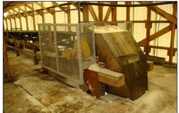
*Note compactness of 60 HP internally-powered hermetically sealed Rulmeca Motorized Pulley drive.*
