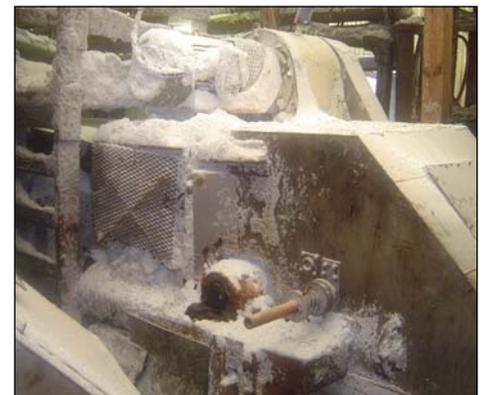
*Note pillow block corrosion and plugged motor cooling fins above conveyor discharge chute before conversion to Motorized Pulley*
