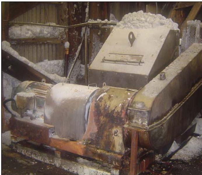
*Original exposed motor, gearbox, chain/sprocket assembly*
